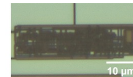
Smallest-ever CMOS biosensor · 40 \mu\text{m}
